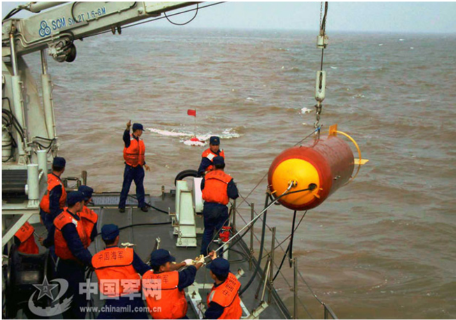
Photo 12. Minesweeping Exercise. Crewmembers on a PLAN East Sea Fleet mine countermeasures ship handle a towed noisemaker used to sweep acoustically triggered mines in May 2008. Already in the water is a marking buoy. Mine rails are visible on the deck to the right of the crane.
